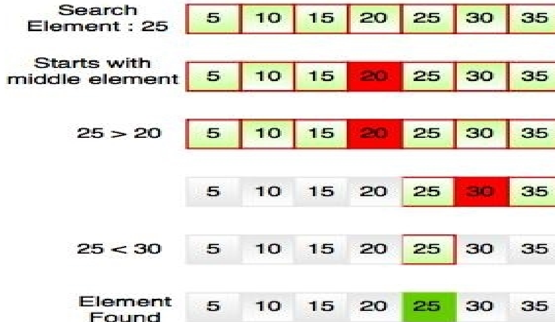
Fig. Working Structure of Binary Search
